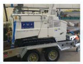
Our purpose built trailer enables easy delivery and collection of the built to the work site, and the Vac-Ex unit to tow along tools or compressor units, whatever the job requires. The remote control unit epitomises non invasive excavation.
