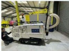
The combination of the powerful vacuum system along with an air lance attachment for agitation ensures all ground can be excavated safely, cleanly, with zero HAV's and a zero strike risk. A perfect non invasive tool for the removal of dust, dirt, sludge or slurry. The machine empties quickly, cleanly and remotely, enabling efficient job completion in the toughest of locations.
